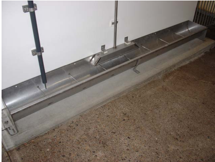
Figure 3. Feed troughs used in the liquid feeding system at the University of Guelph. The height of the concrete pad underneath the feeder varies from 1" on one side to 4" at the other side to correct for slopes in the floor.
