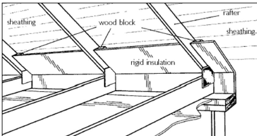
Figure 3: Insulating the outside edge of the attic floor
