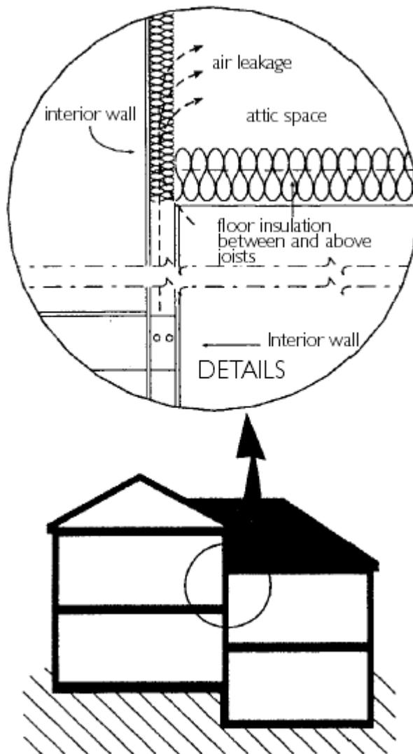
Figure 2: Leakage areas on split level houses
