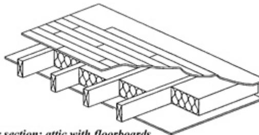
*Floor section: attic with floorboards*
