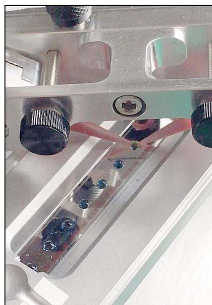
**Figure 3.** Strider™ fluid head applies measured fluid droplets directly to samples in succession. A subsequent fluid head washes this fluid droplet away, after which the sample air-dries and then respoos onto a pickup reel.
