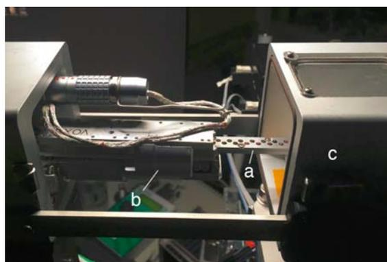
**Figure 1.** GridStage Sprite™ cartridge-based sample stage. Sample carrier cartridge (a) holds sixteen 3mm grids and is mounted onto (b) stage body comprising multi-axis positioners. Stage body is mounted into a load lock (c) that automatically inserts it into microscope to the right (not shown).
