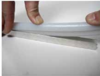
Figure 10: Push the tube into aluminum mount
