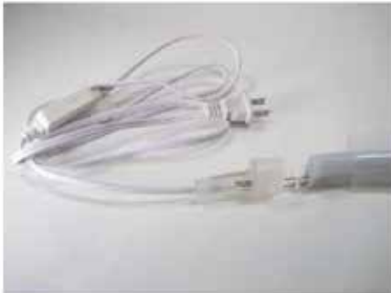
Figure 1: Connect Power converter to tube
