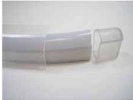
Figure 8: Put the end cap on the end
