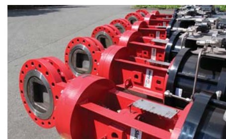
Variable orifice gate style control valves are ready for slurry service.
