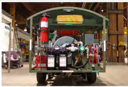
This is the rear view. Here is the fire extinguisher, the spill kit, the two filter housings, as well as the fuel/defuel valve and pre/post filter fuel sample ports. This is also where the tire/strut hose reel is mounted.
