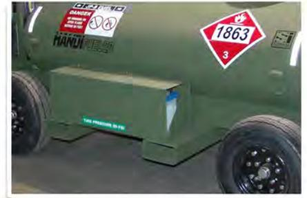
Close-up view of battery box that houses two Optima deep cycle batteries, the fork lift pockets and the heavy-duty tie down lugs.
