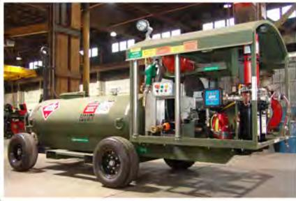
Operator's panel with access to controls, meter fuel log stowage, grounding reel, and fuel nozzle. Notice the two vertical stainless steel hose guides.
