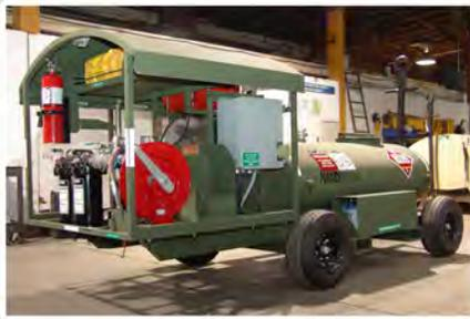
Right side where we find the weatherproof electrical box that houses the charger. Also here is the stowage area for oil/hydraulic fluid or the optional SPR nozzle. Note the NATO plug on the electrical box.
