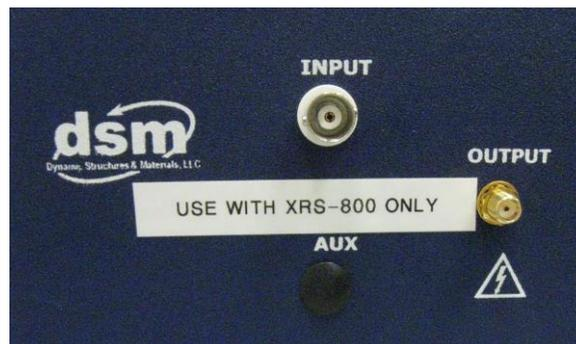
*Input and Output Connections on Front Panel of VF-500-XRS with Waveform Generator calibrated for an XRS-800 stage*
