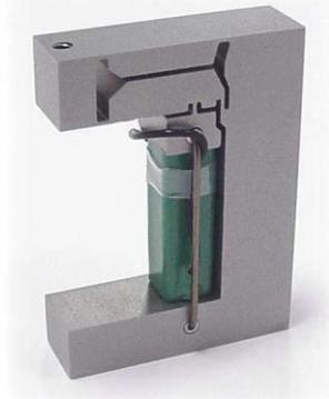
Figure 3 – DSM LPA-100 piezo actuator uses a simple lever-arm mechanical amplification. (PZT stack is green - output is in vertical direction)
