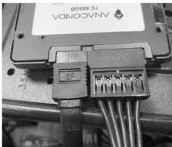
SATA connectors used for hard drive, CD-ROM and cooling fans.
