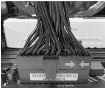
Plug the 24-pin connector onto the motherboard.
