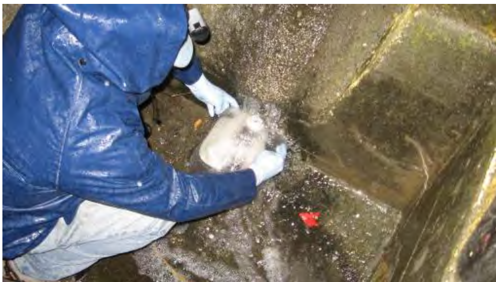
Collecting a sheet flow stormwater sample.
