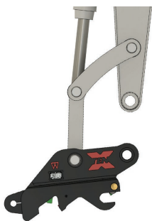
Fig. 3.4.1 Raise dipper arm to take weight off coupler
