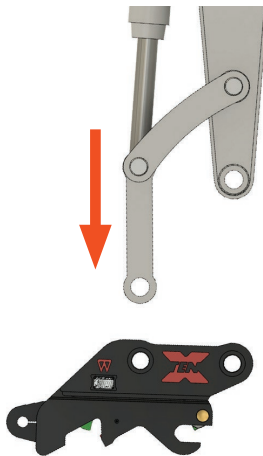
Fig. 3.3.1 Lower linkage into coupler
