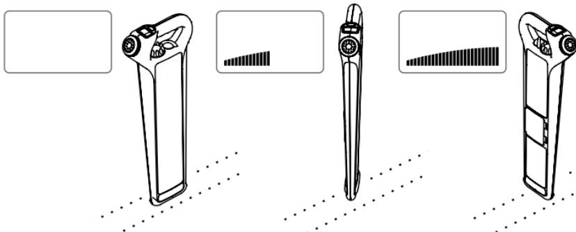
Trace the buried conductor keeping the C.A.T4 vertical and moving it steadily from side to side. Follow the line of the buried conductor, marking it as required across the area to be excavated.
