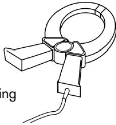
Plug the Clamp into the Genny4 accessory socket. Place the Clamp around the pipe or cable ensuring the jaws are completely closed. Switch the Genny4 on then open and close the Clamp. If the jaws are closing correctly there will be a change in tone as the jaws are closed.
