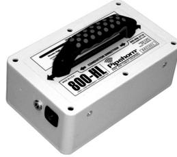
**During Inductive Mode** only the High-Frequency is being induced. To put the most signal on a conductor, place the handle of the transmitter in-line and directly over the conductor.
