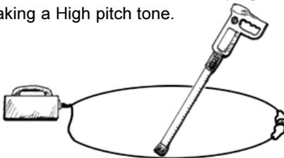
If the Receiver volume is low replace the batteries. If your Pipehorn does not perform as above, replace batteries and try again. Otherwise it may be in need of service or calibration.
