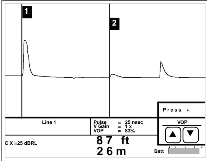
The middle reflection at the 2nd cursor is a partial open followed by a complete open (end of the cable). The more severe the fault, the larger the reflection.
