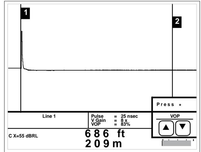
A properly TERMINATED cable will absorb the TDR signal, resulting in no reflection. Faults prior to the termination may appear as reflections along the waveform.
