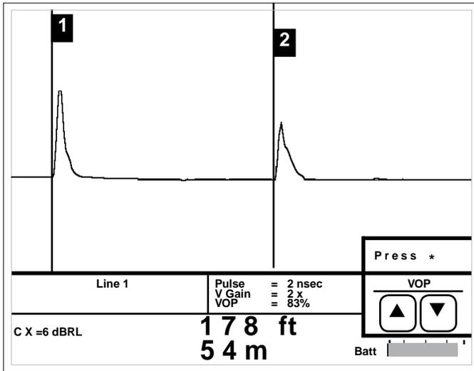
A reflection with the same polarity indicates a fault with OPEN (high impedance) tendencies. The reflection shown at the 2nd cursor is a complete open.
