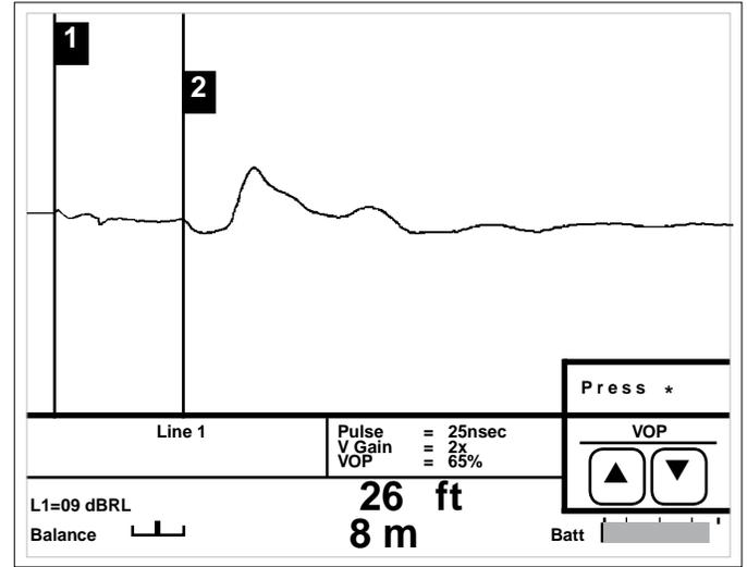
A wet splice at the 2nd cursor. This is the first splice out from the cross connect.
