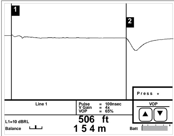
A reflection with downward polarity indicates a fault with SHORT (low impedance) tendencies. The reflection shown at the second cursor is a DEAD SHORT.
