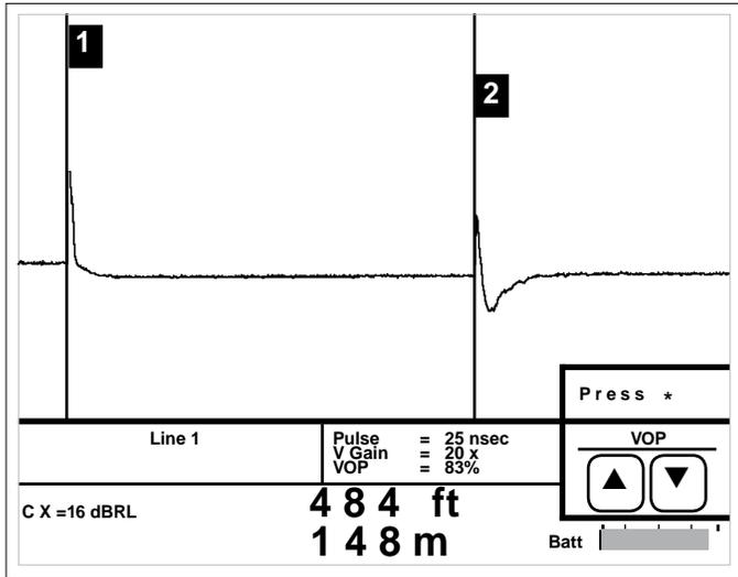
Testing through to an antenna usually results in a “S” shaped reflection, although reflections can vary greatly depending on the antenna.
