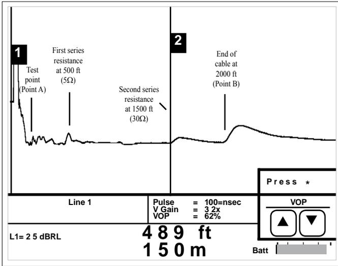
After the first major reflection, the second event could be a more severe fault. It appears smaller due to absorption of signal at the first fault. Always test the cable from both ends to help eliminate this problem.
