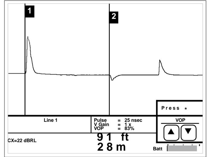
The middle reflection at the 2nd cursor is a partial short followed by a complete open (end of the cable). The more severe the fault, the larger the reflection.
