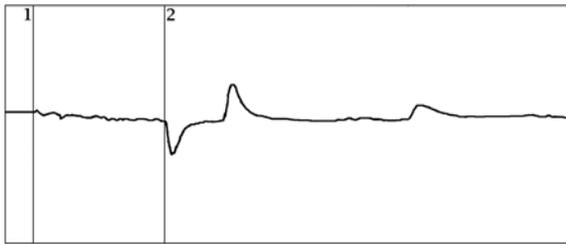
The distance between the two cursors is the distance from the TDR to the point of the bridged tap.
