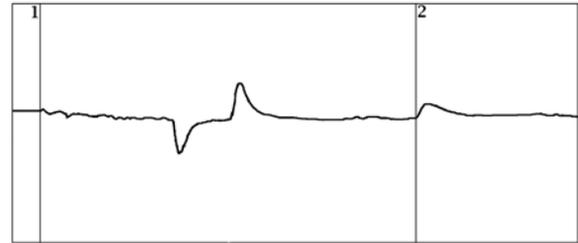
The distance between the two cursors is the distance from the TDR to the end of the main cable. There is no need to subtract the length of the lateral. This is an advantage of a TDR over an *open locator*.
