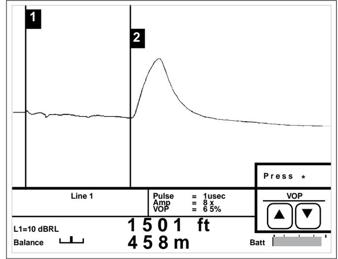
A telephone load coil will cause a high impedance UPWARD reflection (similar to a COMPLETE OPEN).
