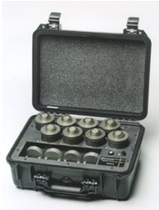
Eight ZCorr loggers are held in a compact *Docking Station*, which is connected to a PC. The docking station communicates with the ZCorr loggers electronically, without cables.
