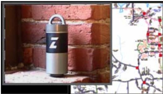
The ZCorr loggers are then deployed in the field in readiness for the nighttime recording.
