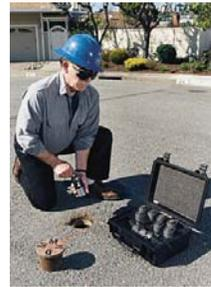
During the night the synchronized ZCorr loggers record at the user-programmed times. Recorded vibration samples are saved in memory. The loggers then enter low-power mode until they are reconnected with the docking station.
