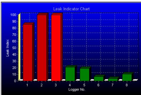
A *Leak Index* (a 0 – 100 ranking) for each logger shows the sound levels present at the quietest time of the night. Each logger is represented by a bar (red = abnormal leak index; green = normal). The listening and sound analysis provide additional capabilities that can supplement the correlation information.
