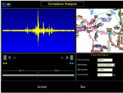
ALFA is particularly useful with large-diameter pipes, multiple leaks, and noisy environments. The graphic above shows a ZCorr correlation result with 6 correlation peaks, identifying 6 leaks in and outside a 530-foot recording span.
