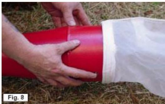
Figure 7 - Installing the exhaust bag.
