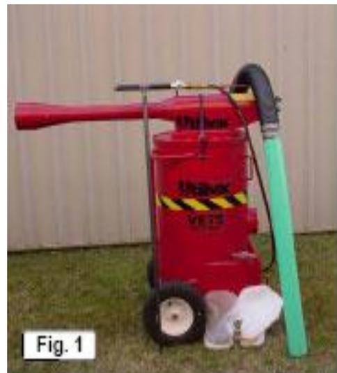
Figure 1: Basic system components: hopper, vacuum generator, control valve, pickup hose assembly
