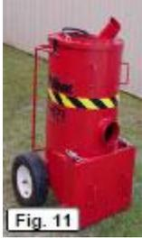
1. Select the appropriate location for the hopper and place it on solid level ground. Ideally the hopper should be about 6' (2m) from the excavation. Check the wheels if necessary to stabilize the hopper. (Figure 11)
