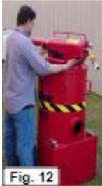
2. Install the vacuum pump so that it points away from persons in the area. Be sure that an exhaust bag is securely installed. Secure pump with elastic hold down. (Inset) Check all neoprene sealing surfaces (upper lid, lower door) for snug fit. Damaged seals or improper attachment will rob system performance. (Figure 12)
