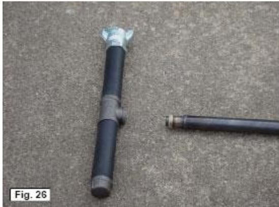
1. To assemble the air lance for use, start by turning the locknut on the lance nozzle or extension barrel as far into the threads as possible. You may need to use a wrench or pliers for this, but do not force the locknut past the threaded portion of the lance or the extension.
