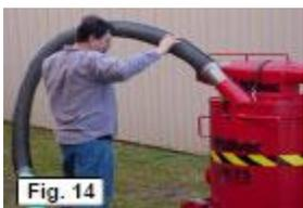
4. Attach the 4' material pickup hose and SDR35. Remember to use the tapered bushing to connect the hose to the gulper tube. The straight bushing is used to connect hose to the hopper. (Figure 14)
