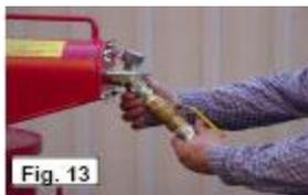
3. Connect the hand operated compressed air control valve assembly to the vacuum generator. Attach hand tight only. (Figure 13)
