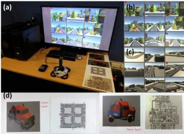
Fig. 7. (a) The Multi-screen system imitates the existing CCTV center. (b) The virtual city and (c) The recreation of the real city in the study. (d) A suspicious truck used in the study for the task, with traditional paper maps provided to the user.
