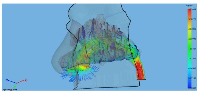
Figure 1: Representation by streamlines of air entry into the nasal cavity. Flow: Inspiration.
