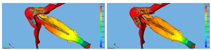
Figure 7: Overview of the outside of the nasal cavity (color map of the pressure field), and streamlines (with color corresponding to the velocity field). Flow: Inspiration. Left: Functional. Right: Virtual Surgery
