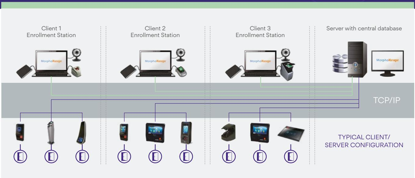
Enroll fingerprint, finger vein/print and 3D facial templates in a single system
