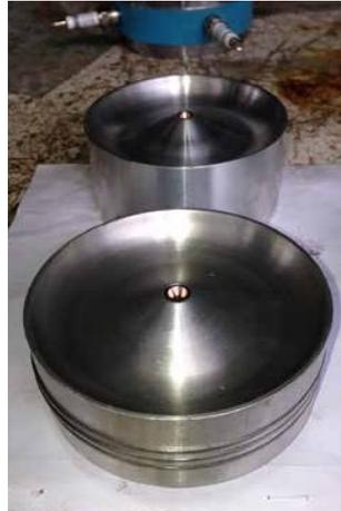
The design for one injector to generate an implosion at the central tungsten carbide sphere.
