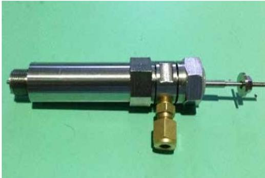
Injector without insulator with fuel and plasmoid inlet
