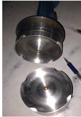
Implosive piston with rings, hydraulic dampener and cylinder head - designed for plasma injector.
