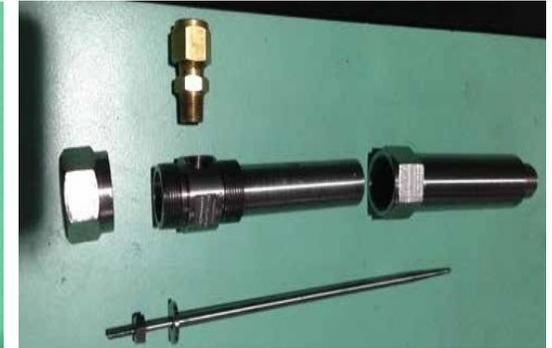
Injector expanded view without insulator or connected fuel and plasmoid inlet
