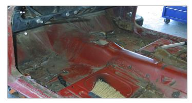
Beware of what you cannot see. This was a floor pan completely covered by carpet. With the carpet removed, it was a shocker. Rust repair is acceptable if the repairs were performed properly. All sheet metal replacement should be performed at the factory seams, not a cut and slice job performed with a cutting torch.
