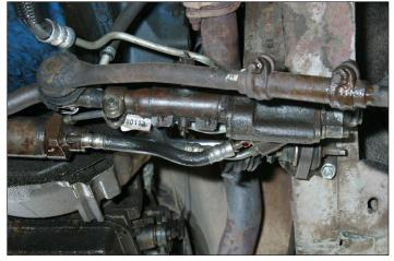
Classic 1965-70 Mustang Bendix power steering is notorious for leakage. Rare is the ride that does not leak. Most of the time, leaks are caused by poor fitting seating. Power ram and control valve leakage are less common.
