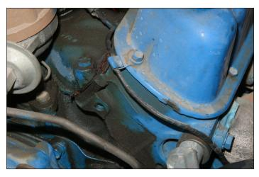
The engine should be free of weepage and leaks that leave spots on the driveway. Excessive silicone sealer like this at gaskets and seals indicates some form of chronic leakage. This is a poor fix with too much silicone.
