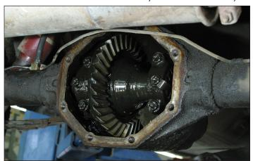
Check condition of differential fluid and listen for noise. Gently lean on the gas and back off listening to the driveline. Lean into the corners and listen for axle bearing noise.
