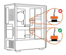
Ensure all component cables are securely connected (some may loosen during shipping). Put the left side panel and screws back on.
