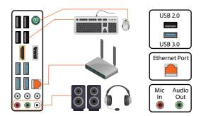
Connect your keyboard, mouse, audio, and network to the matching ports on the motherboard I/O by connection type or color. Any included network adapters or antennas will be in the motherboard box.
