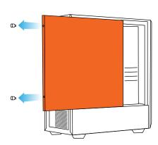
Remove screws from the left side panel. Then remove the panel.
