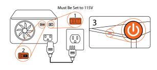
Use the included power cord to connect your power supply unit (PSU) to a wall outlet or surge protector. Turn the power supply switch on before pressing the front power button.
