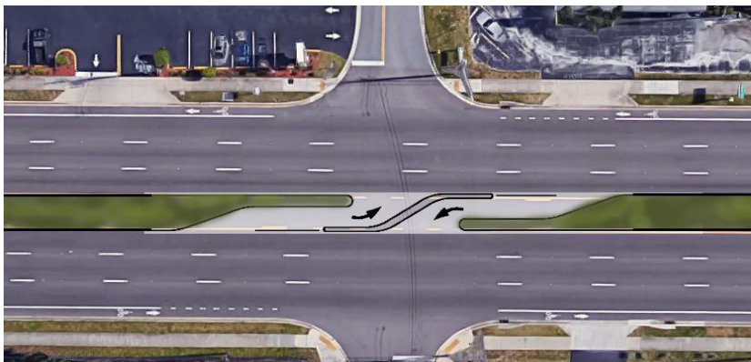
Figure 17: Directional median replacing signal
