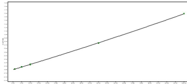
**Figure 3** Representative calibration curve for Propionic Acid (1.00 – 100  $\mu\text{g/mL}$ )
