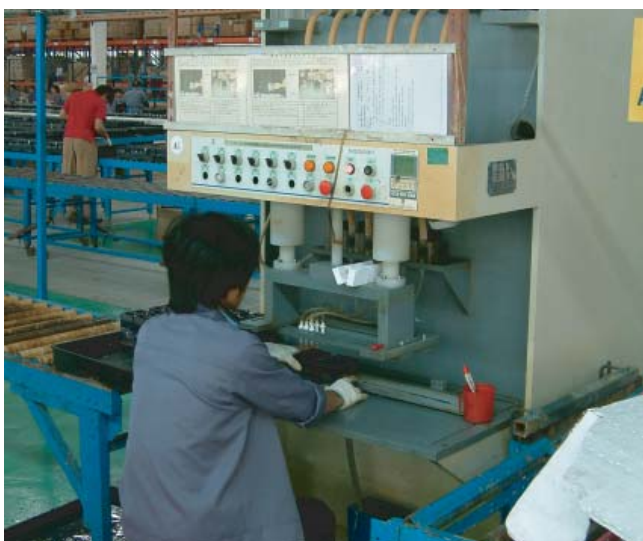
Electrolyte filling of the battery
