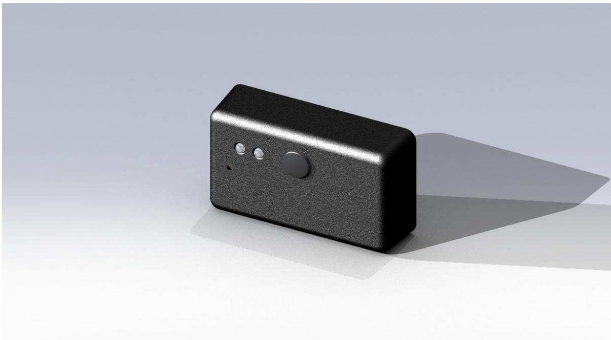
The Wi-Light dongle is a self contained wireless transceiver which can be added to any DMX controlled Photon Beard Hilight fixture. It outputs data directly into the DMX decoder and completely removes the need for any control cable. DMX cable may still be connected but priority is given to the wireless connection. The local manual fader and address setting will continue to work as normal.
