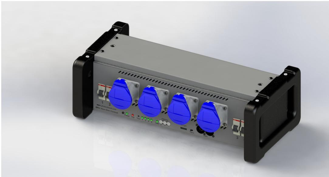
The Photon Beard Four Channel Non-Dim unit is a DMX512 controlled power switching unit. It is intended to supply power to any electrical equipment up to 16A load in response to a DMX control signal. Switching is by relay contacts timed to coincide with zero crossing on the AC supply. Typical applications include remotely powering moving lights, motorised effects or any equipment that may draw current when not in use.
