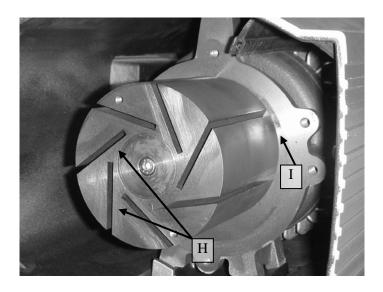
6. Bolt the pump housing back on to the pump.
