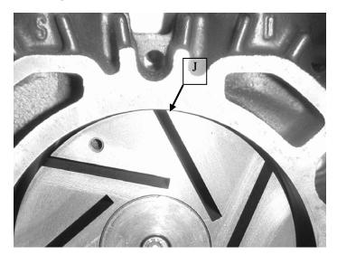
7. Install new vanes. Check to be sure high point in the tapered edge, points in the direction of rotation. Ensure vanes fit freely into vane slots. Reinstall endshield. Install NEW filters and bolt filter housing back onto pump. Start pump and check rotation. The parts required to undertake the replace of the vanes in the T series pumps are in the attached list.
