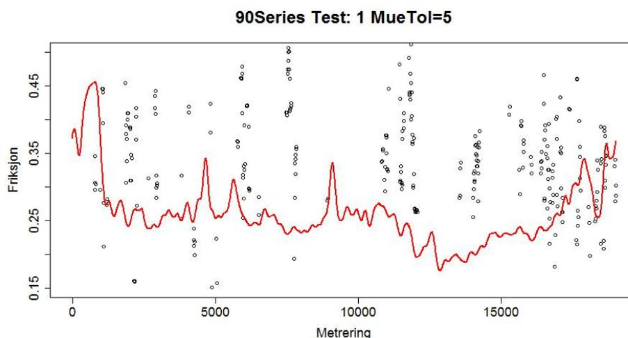
**Figure 5: Comparing measurements from RoAR (red) with friction estimates from the two XC90 Volvo cars with quality higher than or equal to 5.**
