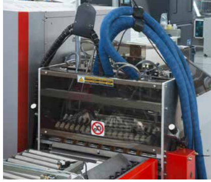
Hot melt application by extruder nozzles
