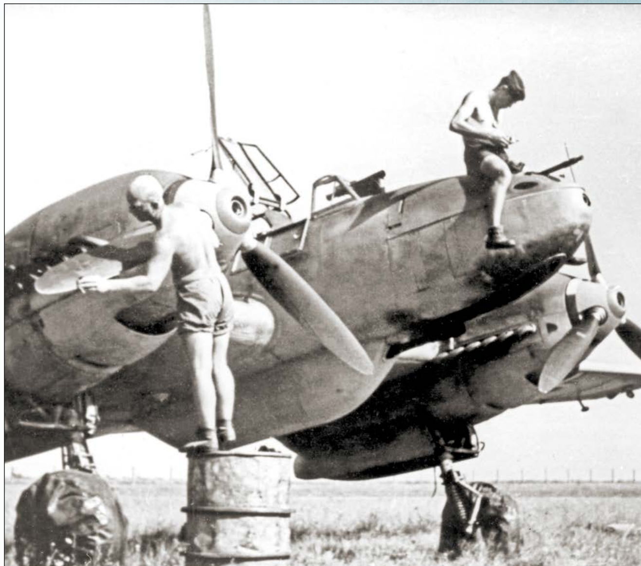
Above: Starboard view of a Bf 110 C-6 showing the fairing that enclosed the 30 mm Kanone.
