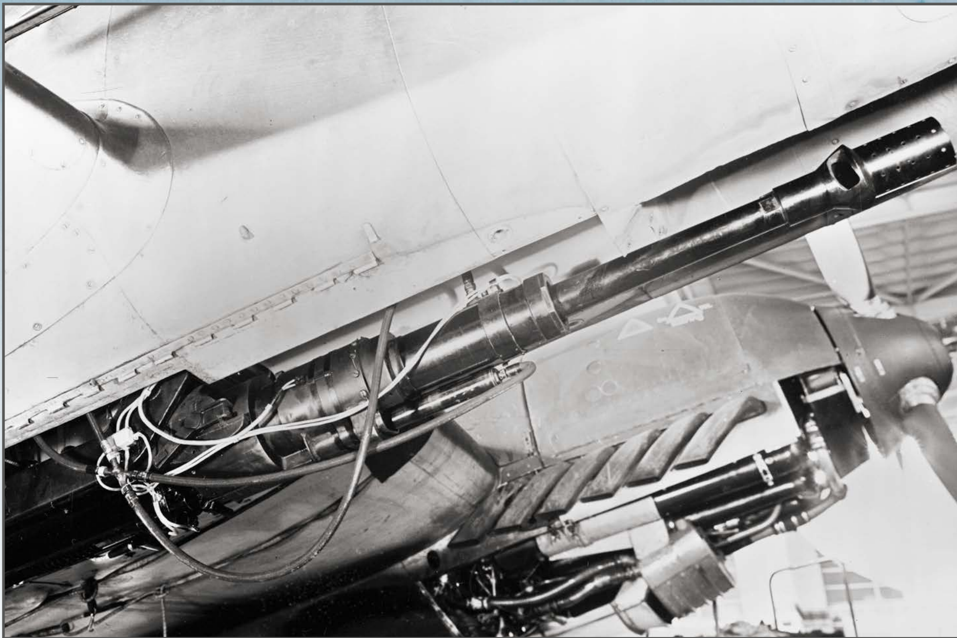
A superbly detailed view of the 30 mm Kanone in place in the fuselage of a Bf 110.
