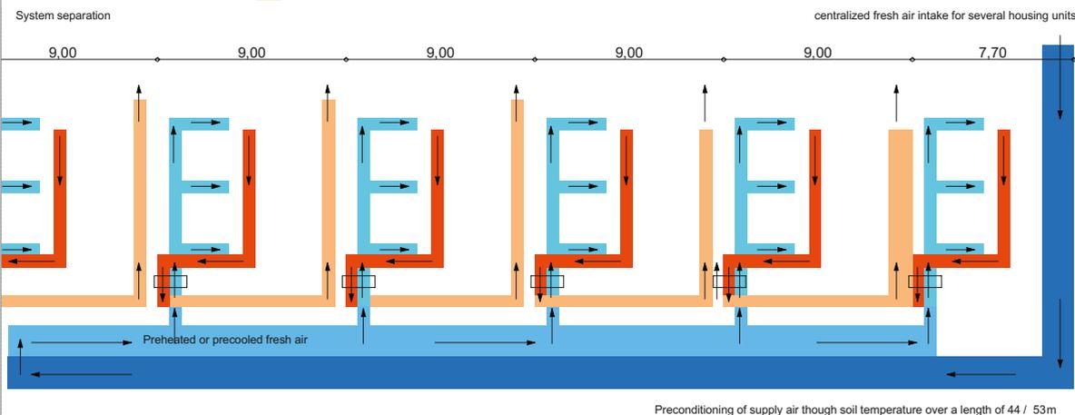
Fig. 8 Earth tube register in an urban unit (Wolpert, A.)
