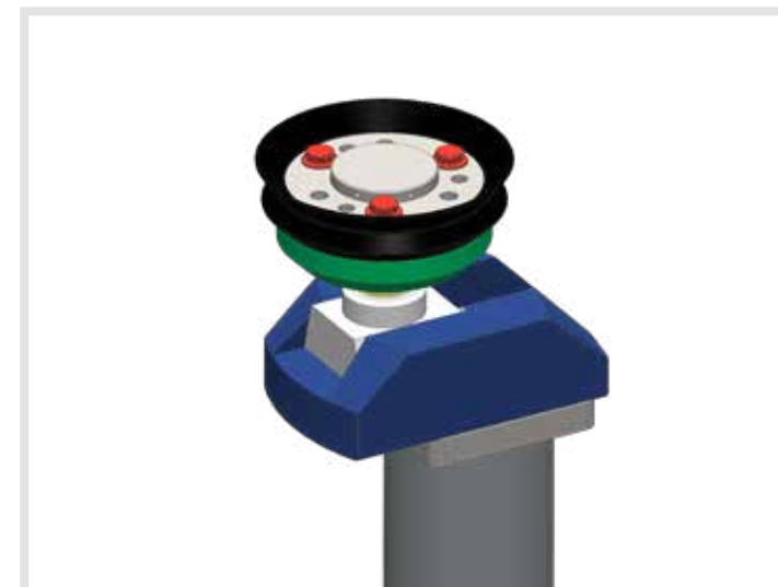
XY adjustment is achieved by sliding end the effector along a dovetail groove in blue offset arm.
