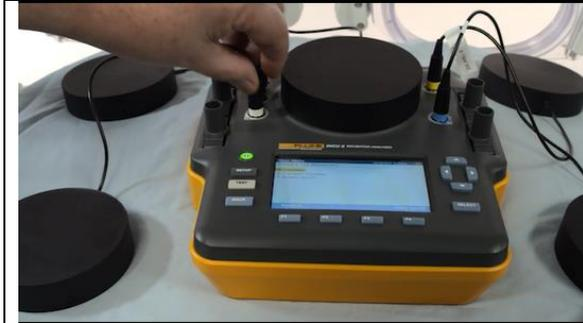
To test radiant warmers, simply replace the temperature probes with the radiant pucks, position them around the warmer according to the standard. Select the appropriate test and testing environment, or use the General Testing feature.
