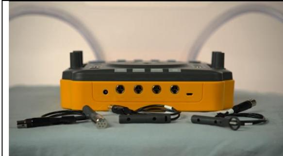
The sound, air flow, and humidity probes plug in the back.
