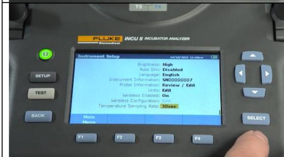
To navigate around on the device, use the navigational arrow keys to highlight a field/test option, and the "SELECT" button to select it. Keys F1-F4 are used to select options on the bottom of the screen. The "BACK" button takes you back to the previous screen. The "TEST" button starts the test. The "SETUP" button (shown to the left) allows you to change your measurement units, sampling interval, and enter or view device details and information.
