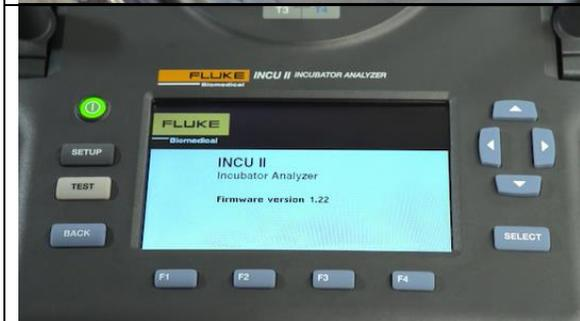
The INCU II has a large LCD screen, on which you will be able to see real-time data and test results. When you first turn on the INCU II, it will do a self-check. When it's ready to test, the main menu will appear.
