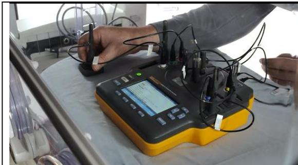
Once the device has been set up and placed in an incubator (shown) or radiant warmer, remove and setup the temperature tripods and sensors. T1-T4 should be in the center of each quadrant of the mattress using the removable tripods, and T5 goes in the middle. There is a colored grid below the device that helps show the proper placement. The sound, humidity, and airflow probes fit into the remaining three slots in the center of the device.
