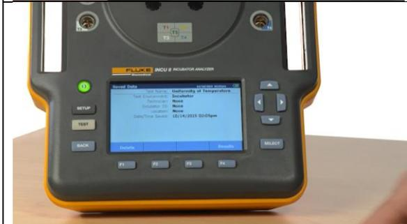
The INCU II will display test data in real-time on the screen—for both the standard tests and the general testing option. If you’re using a standard test, a pass/fail indicator will be displayed at the end of a test.
