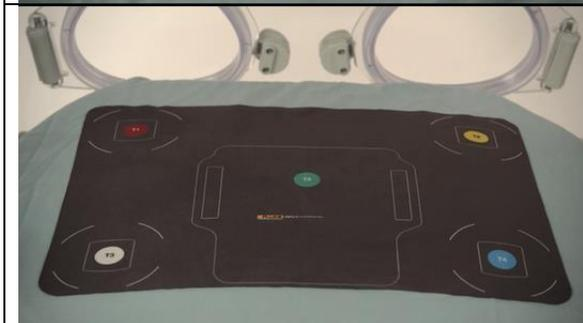
The placement pad is laid in the incubator/radiant warmer and helps ensure the placement of the probes for more accurate measurements. You can use this as a guide to find the center of the mattress and the center of each quadrant—but remember that these points will differ slightly for different mattress sizes.
