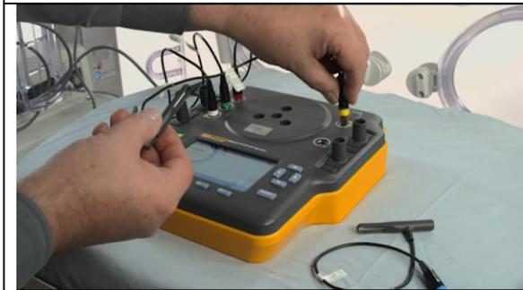
To begin, plug in the probes for the parameters you want to test. This can be done either before or after the device is placed in an incubator/radiant warmer, but is easier if it is done beforehand.
