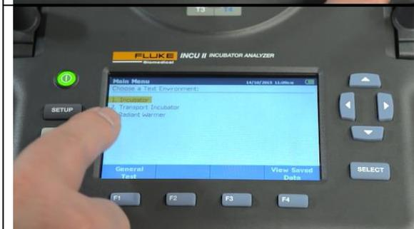
This is the main menu, showing: Select a Test Environment, General Test or View Saved Data.
