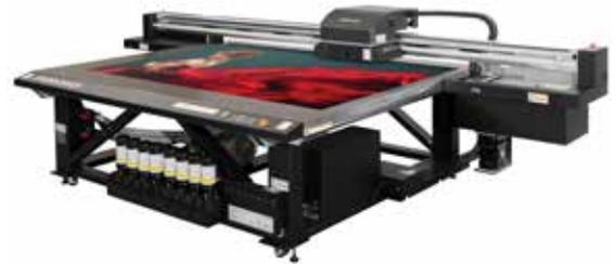
This innovative printer adds new productivity and functionality to our proven JFX200 technology. It also adds extra dimension to graphics with an advanced 2.5D Print Function that lets you create realistic textured effects up to 0.5 mm high - with the touch of a button.
