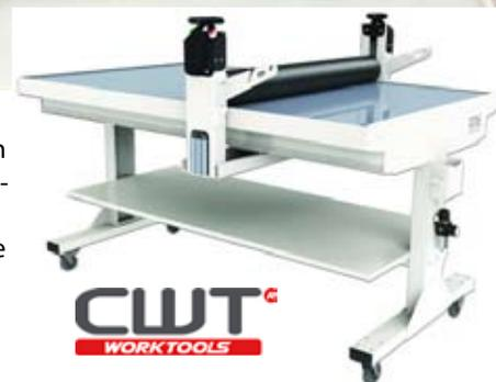
The CWT Worktable solution is one to pay attention to. This table can apply laminate or transfer tape, it can mount prints to boards, and it can do it all with the push of a button and the smooth roll of a foam wheel.
