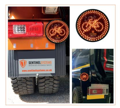
The LED Cycle Sign is designed to warn and prevent vulnerable road users from going down the nearside of the vehicle. Connected to the nearside indicator, the sign will illuminate when the lorry signals to turn left when travelling at low speeds.
