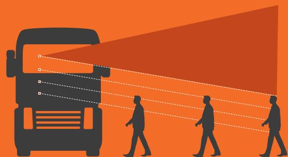
**DIRECT VISION OBJECTIVELY MEASURES A DRIVERS VIEW THROUGH THE WINDOWS OF AN HGV CAB**
