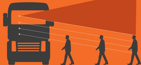
**DIRECT VISION OBJECTIVELY MEASURES A DRIVERS VIEW THROUGH THE WINDOWS OF AN HGV CAB**
