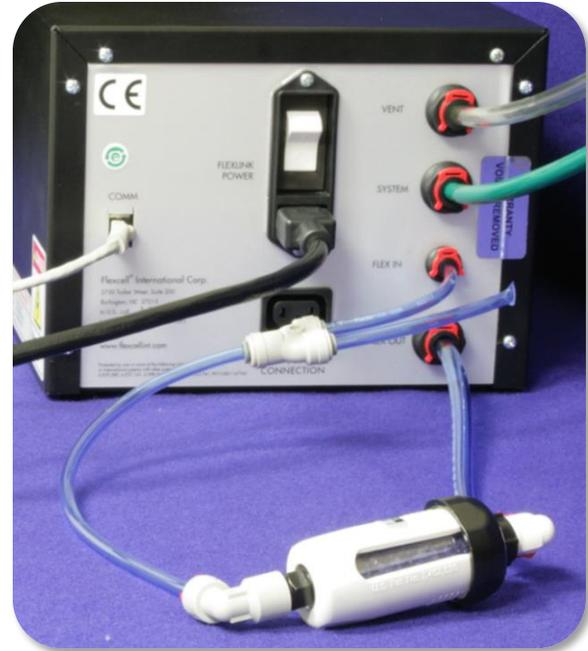
**Figure 6.** Setup of a drying filter in-line with an FX-6000™ Tension System.
