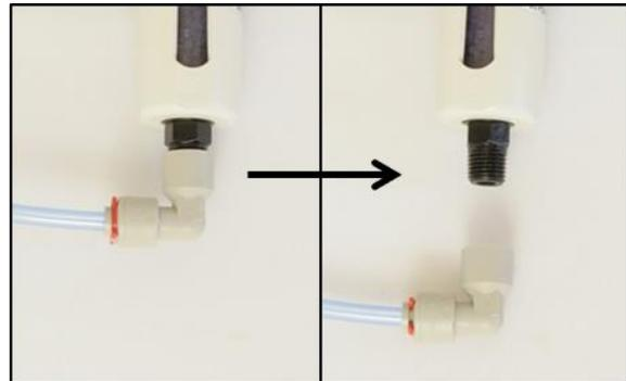
**Figure 8.** Remove  $\frac{1}{4}$ " tubing connector.
