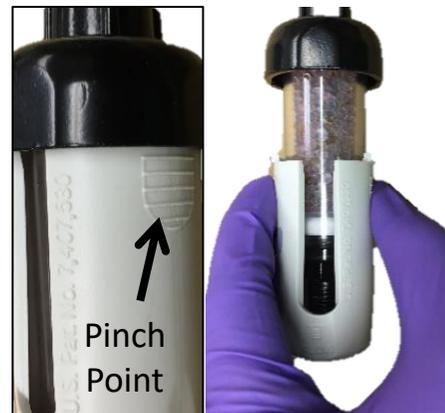
**Figure 9.** Remove plastic housing.
