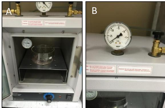
**Figure 11.** A) Saturated desiccant beads in drying oven. B) Drying oven with vacuum set to -29 in Hg.
