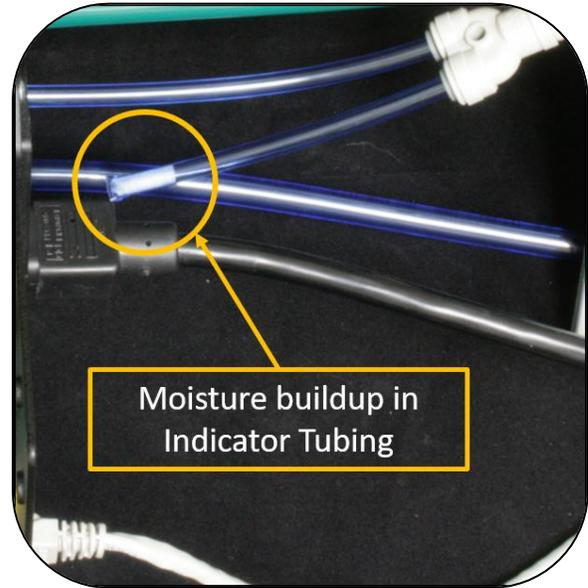
**Figure 4** - FLEX IN moisture indicator tubing with visible moisture accumulation
