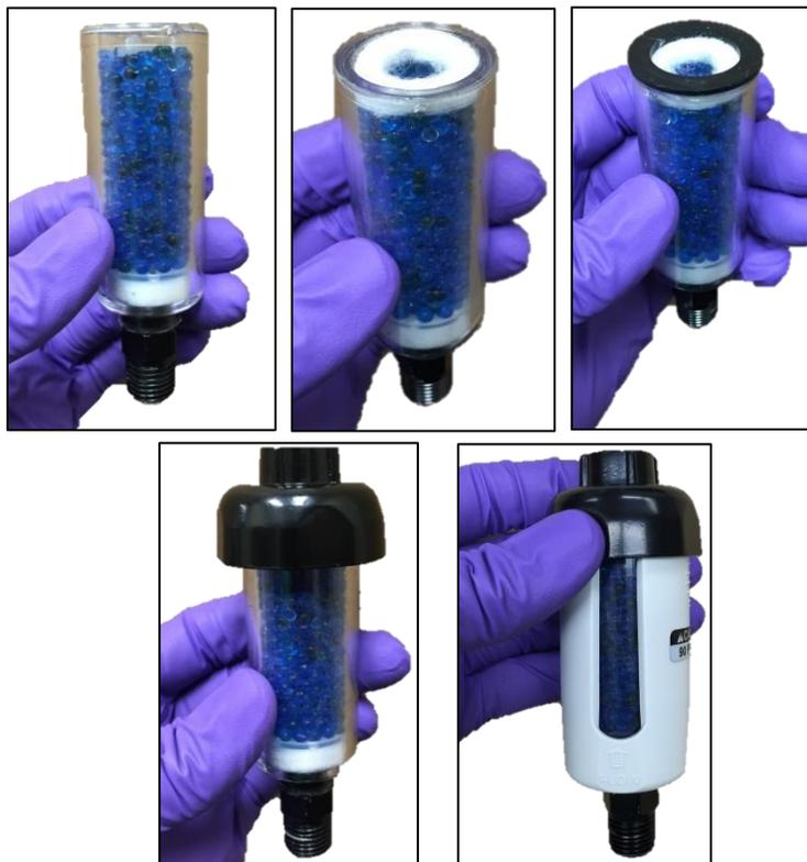
**Figure 14.** Re-assembly of drying filter.
