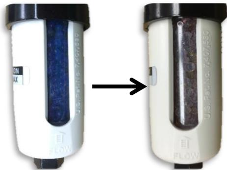
**Figure 7.** Drying filter ready for use (left) and saturated drying filter (right).
