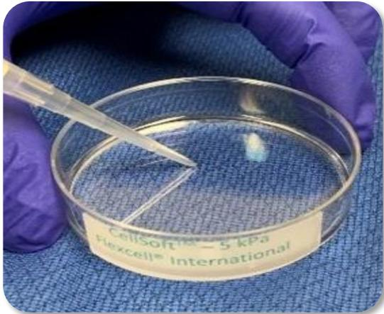
**Figure 4.** CellSoft® substrate (5 kPa stiffness silicone elastomer polymer) in the 100 mm diameter polystyrene dish Panel A.
