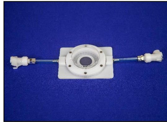
Figure 1. Flexcell®'s StageFlexer I® for use with an inverted microscope objective.
