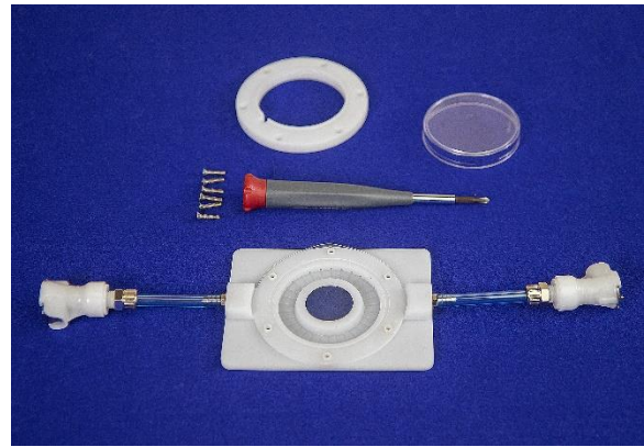
Figure 4. StageFlexer I® device with SFI membrane atop the base.
