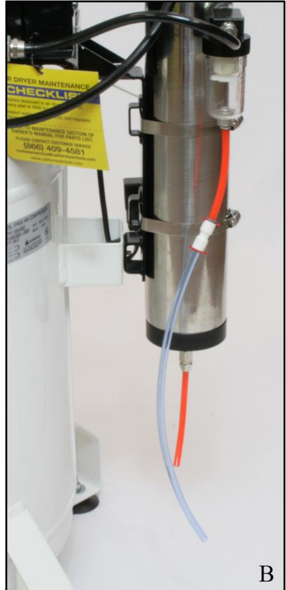
Figure 6B. Extended drain tubing segment from filter bulb
