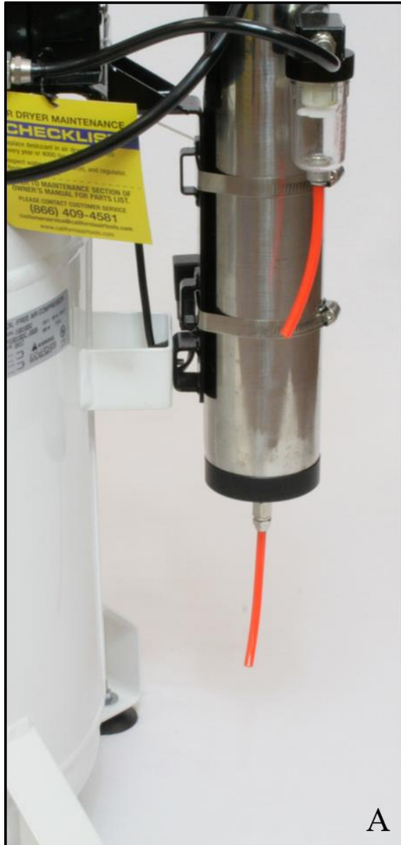
Figure 6A. Drain tubing segments from drying tower and filter bulb
