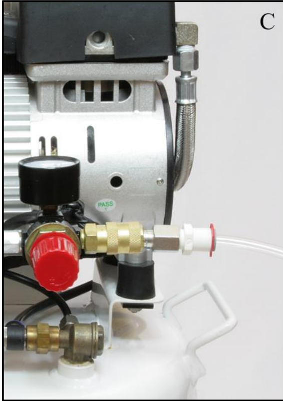
Figure 4C. Compressor Outlet with Zinc Coupling and 3/8" Clear Tubing
