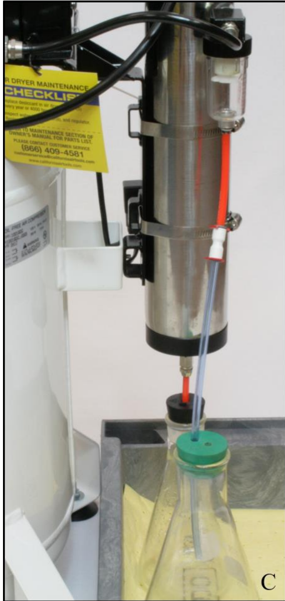
Figure 6C. Drain tubing segments fed into reservoir flasks
