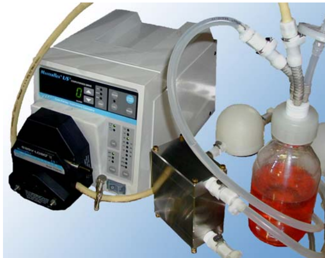
Figure 11. Image of Streamer ® system setup with peristaltic pump, two pulse dampeners, and media bottle.
