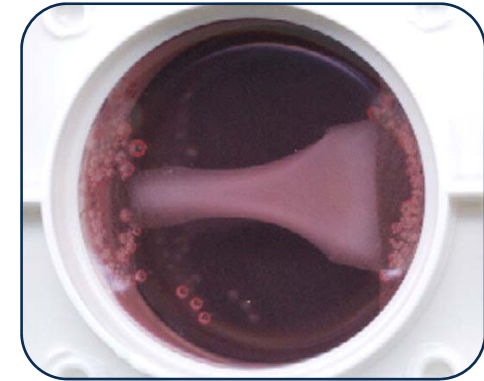
Figure 2. Cell seeded collagen hydrogel in a trapezoidal Tissue Train® culture plate well.
