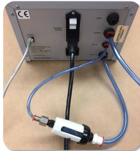
Figure 2. Setup of the drying filter in line with FLEX IN and FLEX OUT tubing and connected to the FX-5000™ Tension System
