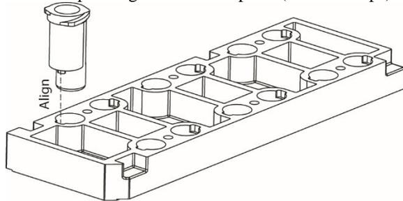
3. Push down the connectors and make sure the contact areas between the connectors and the AIM chips are flush.
