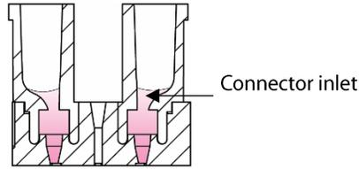
*The media levels should be the same as or slightly above the level of connector inlet*
