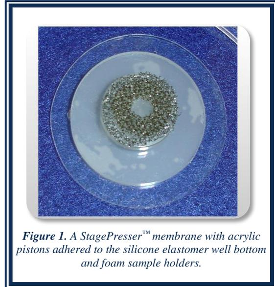
Figure 1. A StagePresser™ membrane with acrylic pistons adhered to the silicone elastomer well bottom and foam sample holders.
