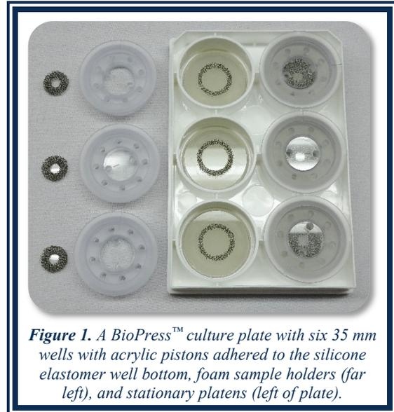
**Figure 1.** A BioPress™ culture plate with six 35 mm wells with acrylic pistons adhered to the silicone elastomer well bottom, foam sample holders (far left), and stationary platens (left of plate).
