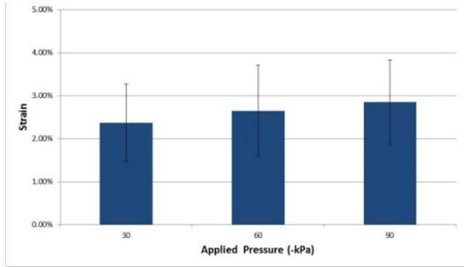
**Figure 2.** Average substrate strain in a HT BioFlex® well when using a 24-well Cell Seeder™.
